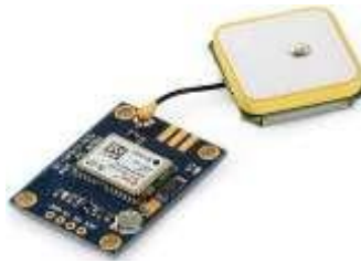
Fig 3. Ublox Neo 6M GPS Module(Source : https://www.nn-digital.com )
