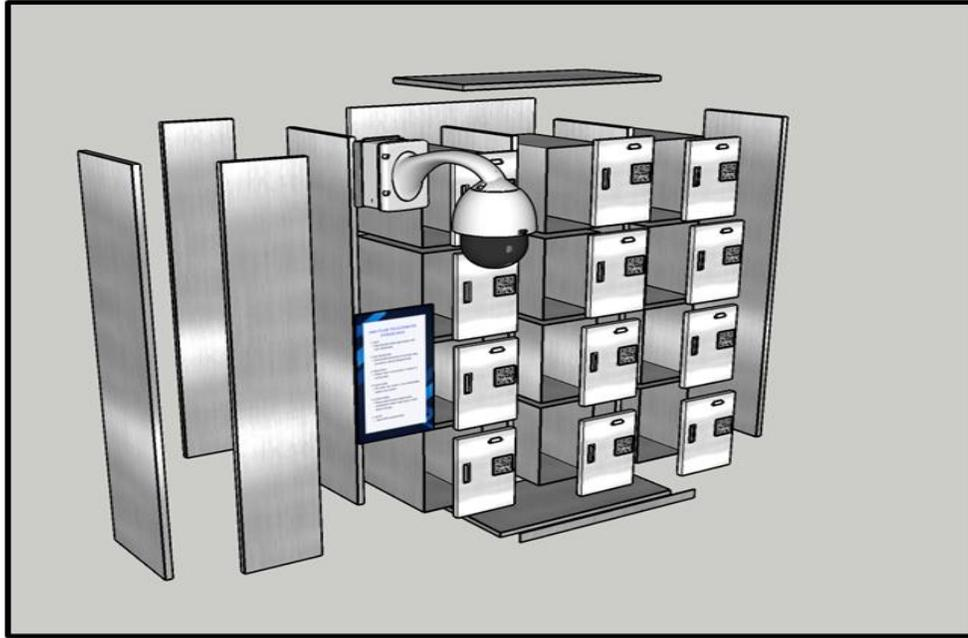
Fig. 2 Exploded View of the Automated Storage Rack
