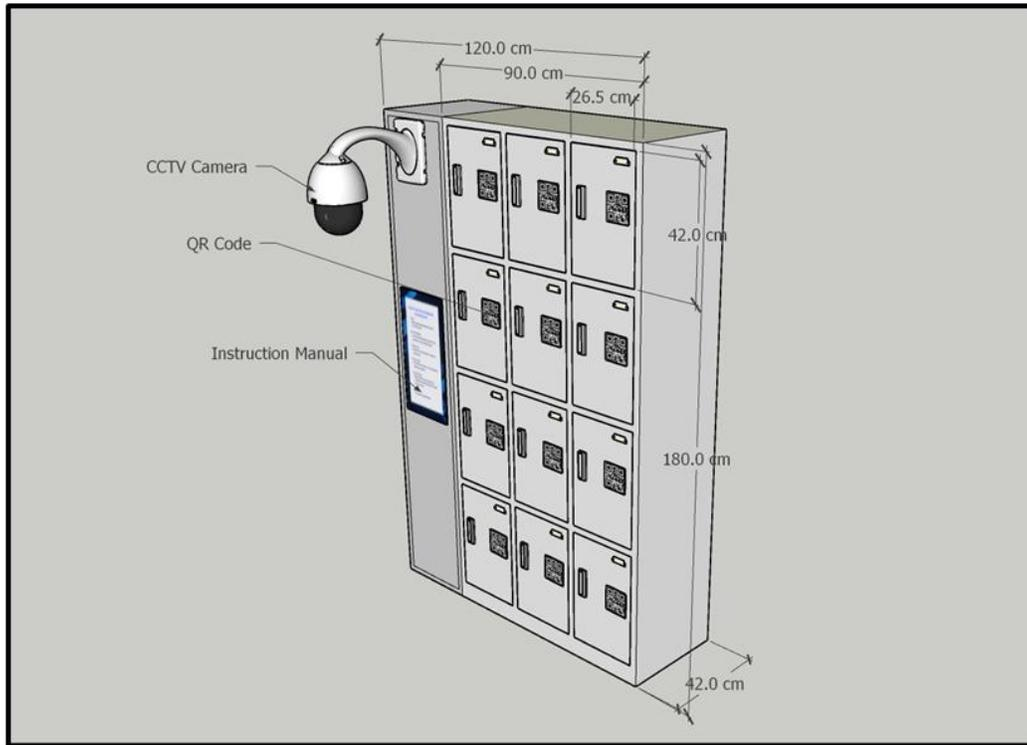
*Fig. 1* Isometric View of The Automated Storage Rack
