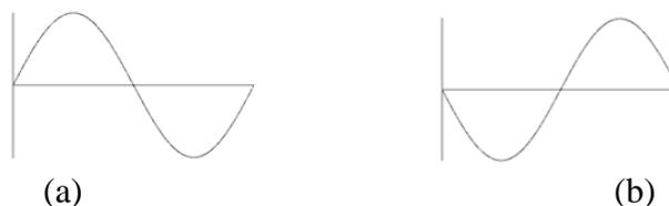
Figure 1. Concept of Noise Elimination, (a) Noise Wave and (b) Anti Noise Wave
