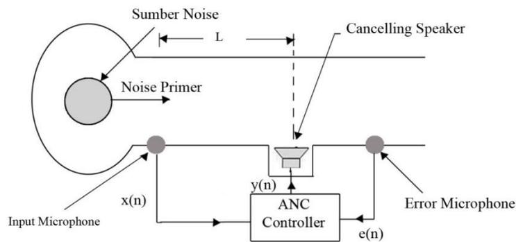
Figure 2. Feed Forward Control
