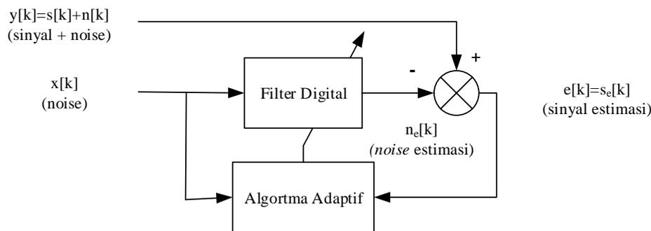
Figure 5. Adaptive Filter Diagram Blok
