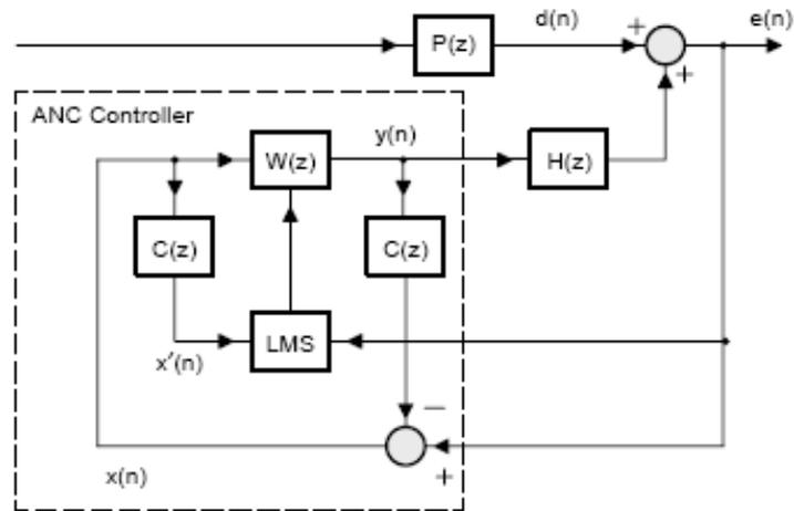
Figure 4. Diagram Block of Feedback ANC
