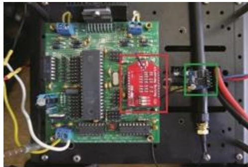
Fig 2. Completely new IoT hardware ESP8266 ESP-05 with antenna (green small square) and old IoT hardware WiFly RN-XV 171 (red big square) placed in low level robot control system (Color figure online).
